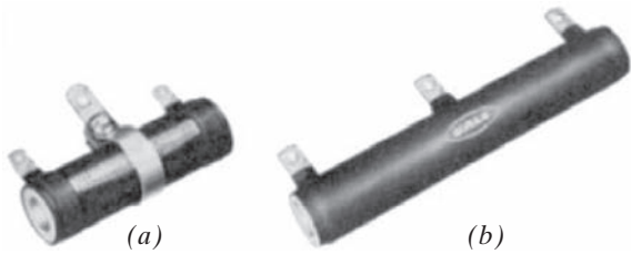
FIGURE 2.4-5 (a) Wirewound resistor with an adjustable center tap. (b) Wirewound resistor with a fixed tap.
